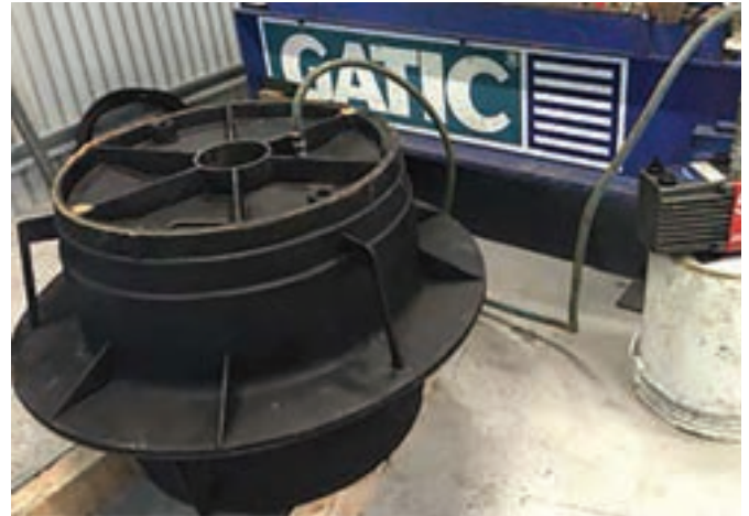
Figure 8: GATIC® EziPit 600 'Top Hat' Cover under vacuum test.
