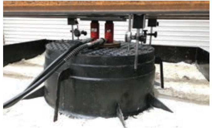
Figure 12: EziPit 1000 MH under load in accordance with ISO Standard 13266
