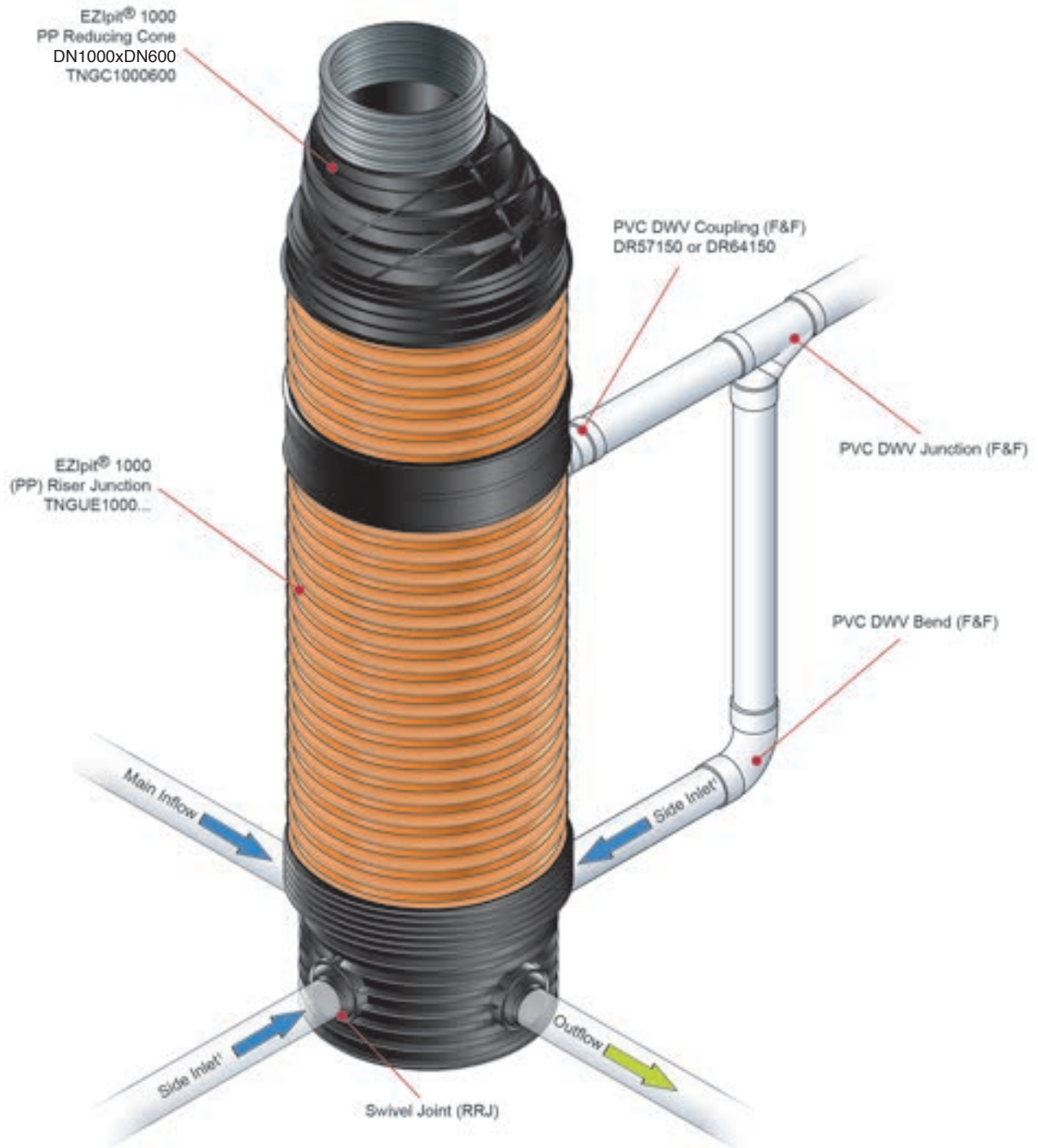
Figure 51: EziPit 1000 Maintenance Hole (MH) with external drop structure
