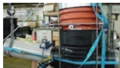
Figure 5: EziPit base and corrugated riser under vacuum test with smooth wall PVC pipes
