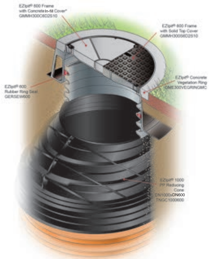
Figure 46: EziPit 1000 MH with GATIC® 'Top Hat' cover arrangement Class B, assembled with reducing cone
