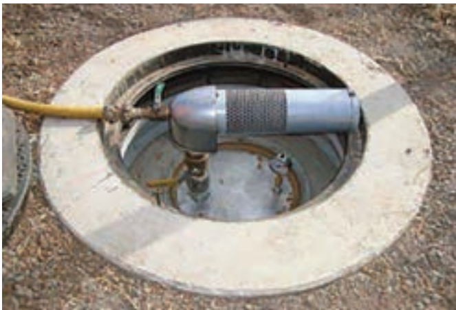
Figure 16: Vacuum test with EziPit test Lid assembled on the Cap and sealed with GATIC® Sealing Compound.
